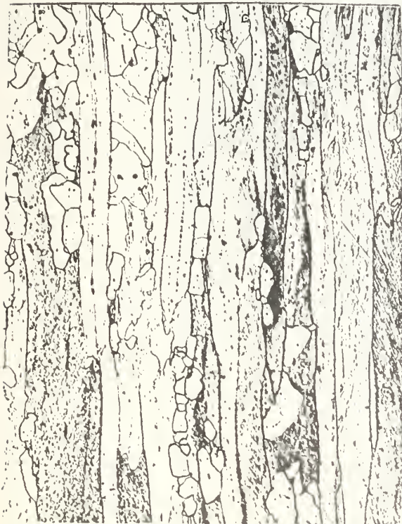
FIG.15 AT 482°C FOR 96 HOURS (ROCKWELL 30T 52.4) -150 X- FIG.16 AT 448.5°C FOR 1242 HOURS (ROCKWELL 30T 52.5)
